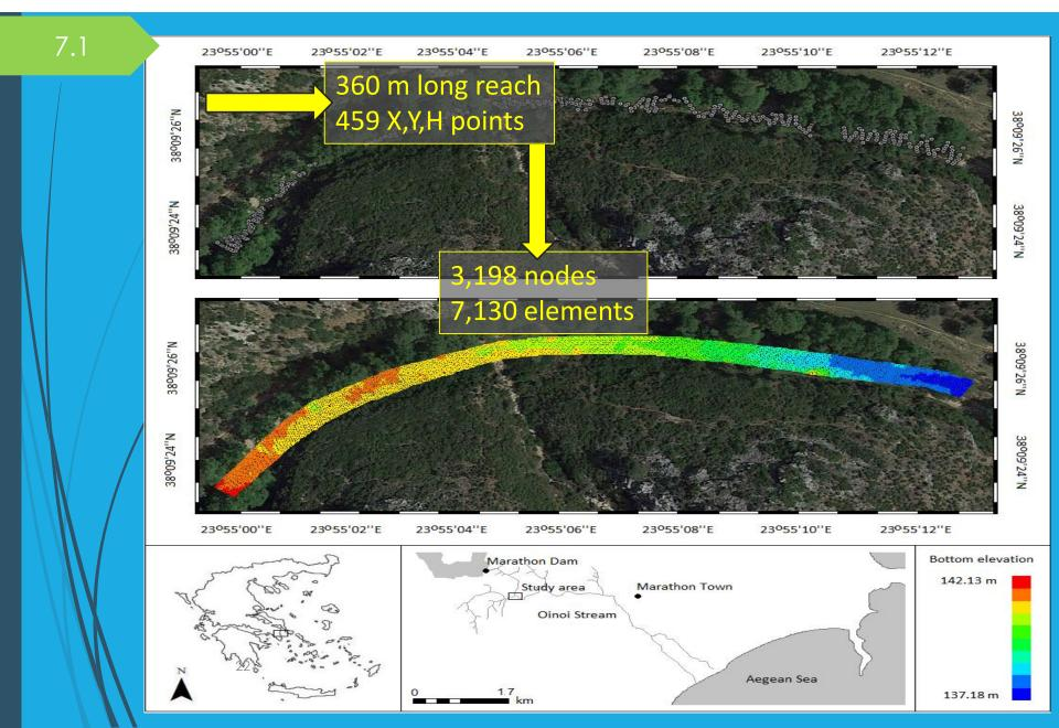
Flow field: adjusting Manning's n in areas based on substrate to achieve max correlation between observed and predicted V and D
